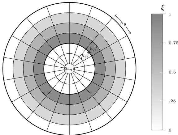
Figure 2: Numerical grid and discretization of the density of microtubules function  $\xi$ .
